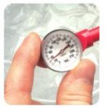
Turn the dial to 32°F. The probe thermometer should have a nut on the underside of the dial. Use this nut to turn the dial, and adjust the reading.
