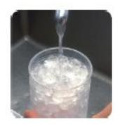
Make a slurry of ice water in a cup. When you fill the cup with ice, add water a little bit at a time, allowing the ice to partially melt. Mixture should be approximately 70% ice, 30% water.
